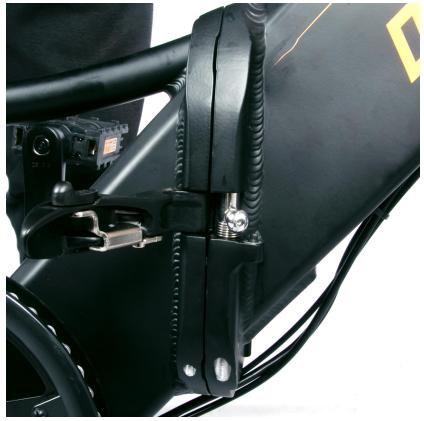
Insert the key clockwise to lock the battery, remove the key and close the frame
