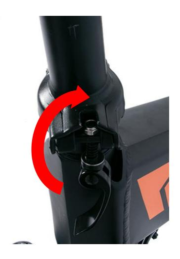
Hold the folding riser upright and the handle of the folding buckle upward to lock the riser
