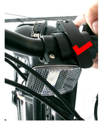
The front reflector is installed
