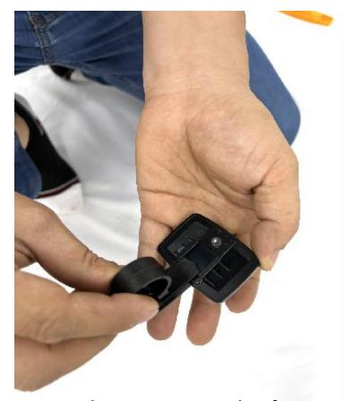
Loosen the screws on the front reflector support using the screwdriver in the tool, and install the front reflector support into the reflector plate along the guide rails
