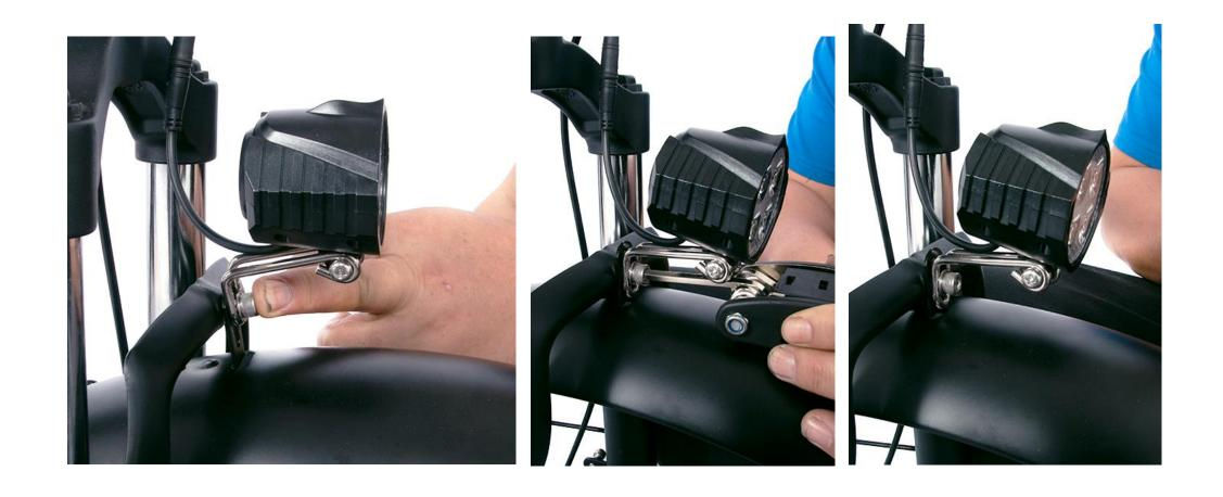
Install the headlight and front fender lifting lug on the front fork with the headlight retaining screws and tighten the screws with the #5 Allen wrench in the too
