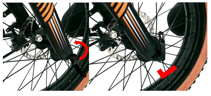
Screw on the quick release rod conical spring nut according to the figure, with the small head of the conical spring facing inward
