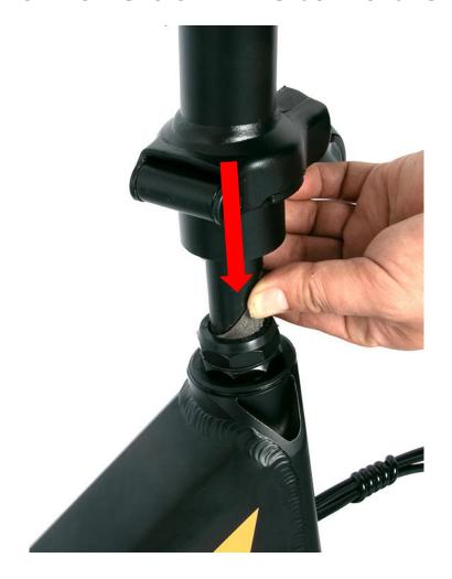
Open the riser folding buckle and insert the riser into the front fork of the head tube along the arrow direction
