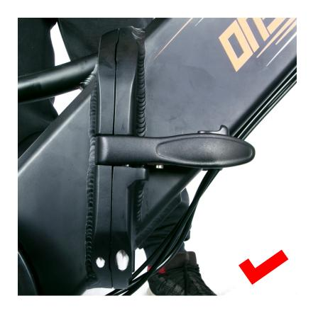
Then fasten the handle of the folding buckle, and the battery is installed successfully
