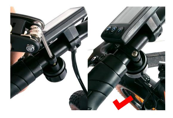
Loosen the screws on the bell bracket using the screwdriver in tool 16 in 1.
