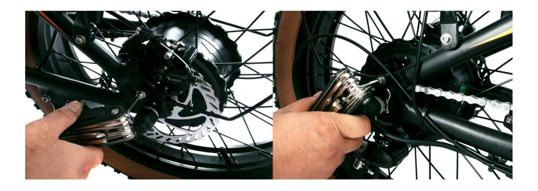
Remove the fender support rod fixing screws and gaskets preinstalled on the left and right sides of the frame with the #4 Allen wrench in the tool, and lock the support rod with screws
