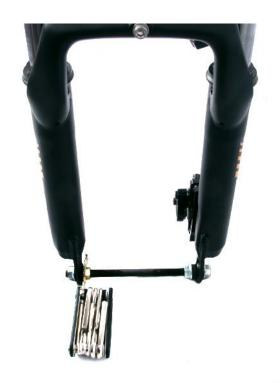
Remove the front fork protection stick with the #15 open end wrench in the tool
