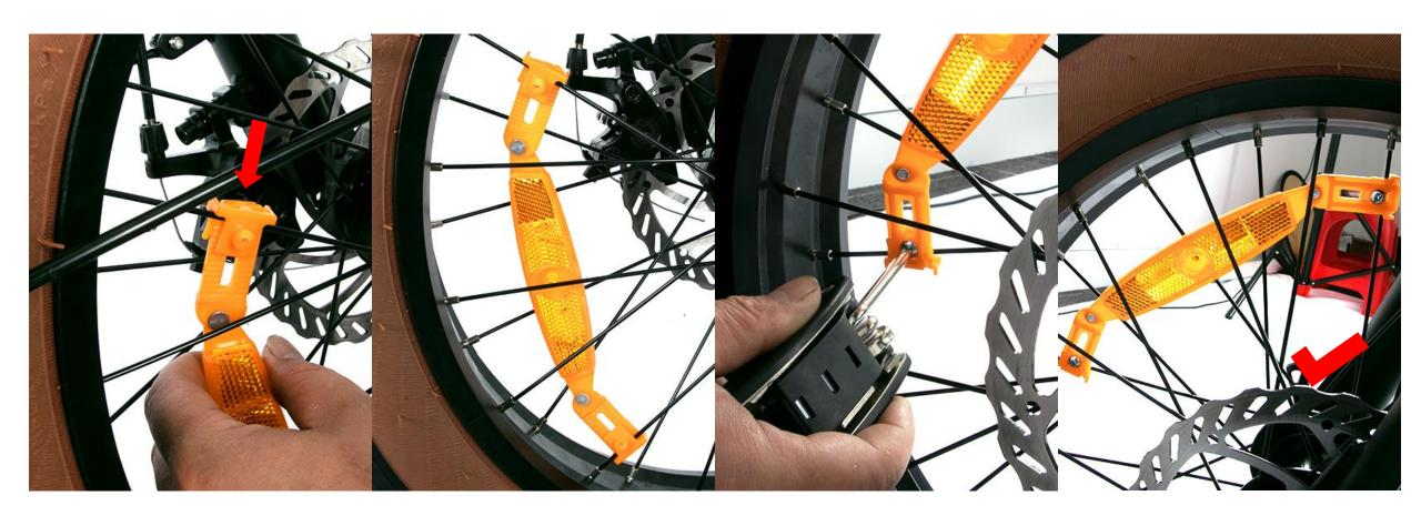
After securing the reflector in the clamp slot, use the screwdriver in the tool to tighten the screws and install the front and rear reflectors
