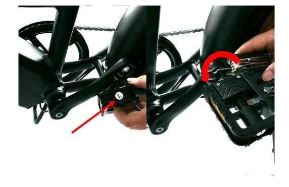
The "R" marked on the foot shaft is the right foot. Rotate the foot shaft clockwise by hand and screw it into the right crank, then rotate it clockwise and tighten it with the #15 open wrench
