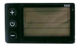
Long press the middle button of the upper instrument to perform the on-off operation
