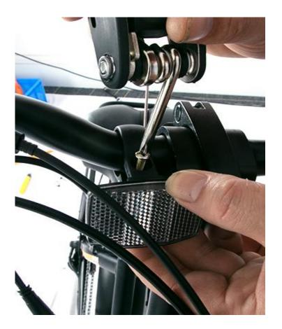
Install the front reflector on the handlebars and tighten the screws with the screwdriver in the tool
