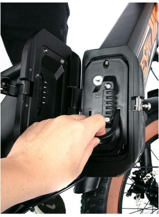
Slide the battery into the battery compartment in the direction of the arrow in the figure
