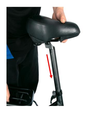
Open the quick release handle of the seat tube clamp in the direction of the figure
