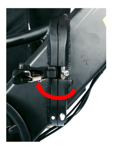
Open the buckle in the direction of the arrow in the figure, and open the buckle outwards
