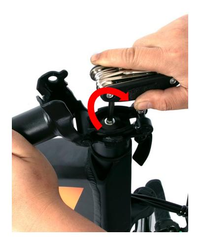
After inserting the folding riser, lock the riser slightly in the direction of the arrow in the picture
