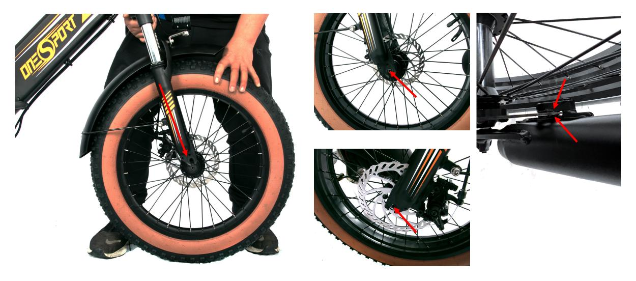
Install the front wheel, the brake pad into the brake to make the gap, the front wheel shaft into the front fork hook claw
