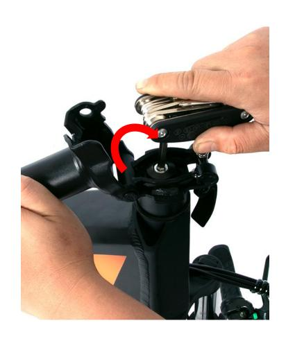
Lower the folding riser and lock the screw in the direction of the arrow in the picture
