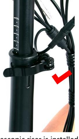
The telescopic riser is installed Note: If the quick release handle is too loose or too tight to move, please adjust the nut tightness properly
