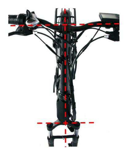
Adjust the handlebars to be parallel to the front fork
