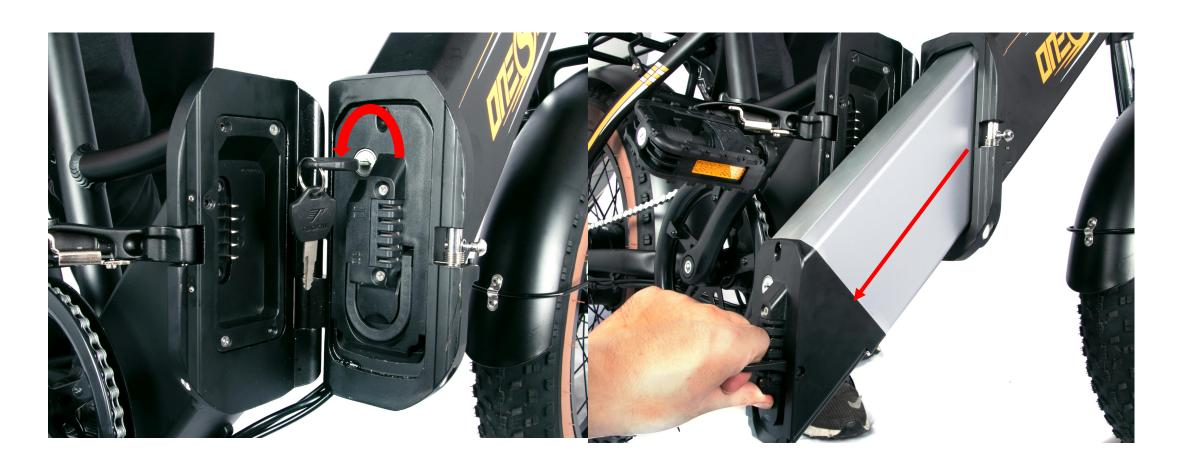
Fold the pipe tube, turn the key counterclockwise according to the figure, open the battery lock and pull out the battery
