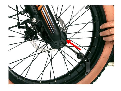
Unscrew the quick release nut of the front wheel and take out 1 conical spring
