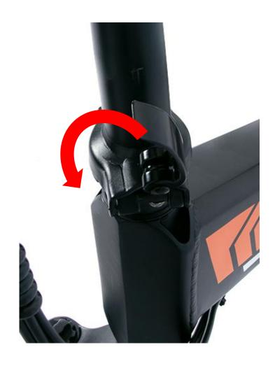
Fasten the handle of the folding buckle in the direction of the arrow in the picture
