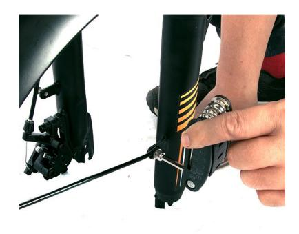
Using the #4 Allen wrench in the tool, remove the fender stick fixing screws and spacers preinstalled on both sides of the front fork, and then install the fender stick tightening screws
