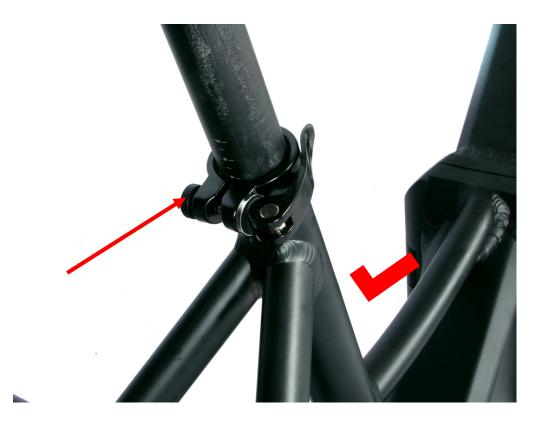
Tighten the quick release nut of the tube clamp, and then fasten the quick release handle of the tube clamp. If the handle is too tight or too loose, please adjust the quick release nut tightness
