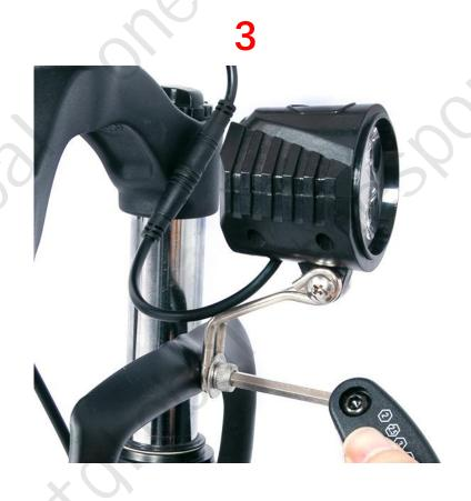
3.tighten the screw with the 5# Allen key in the 16 in 1 tool.
