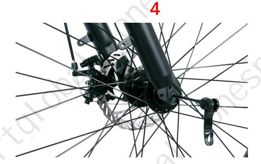
4. Inserting quick release lever.
