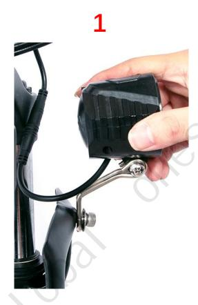
1.Pre install the front light onto the front fork with the fixing screw
