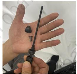
3.Unscrew the quick release rod nut and take out the conical spring.
