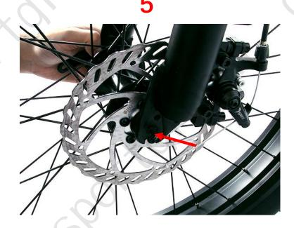
5..Install the conical spring as shown in the figure.
