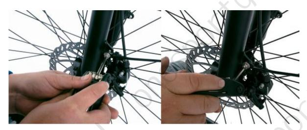
1.Use the 4 # Allen key in the 16 in 1 tool to remove the fixing screws of the pre installed fender support rods on both sides of the frame.
