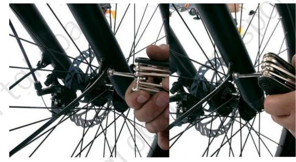
2. Fix the rear fender support rod on the corresponding screw hole of the frame and tighten the screws with the 4 # Allen key in the 16 in 1 tool.
