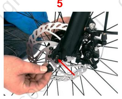
5.Install the conical spring as shown in the figure.
