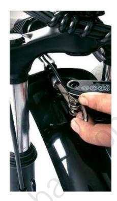
5. Tighten the nut with the assembled tool.
