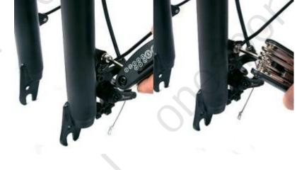
6.Use the 4 # Allen key in the 16 in 1 tool to remove the fixing screws of the pre installed fender support rods on both sides of the front fork.
