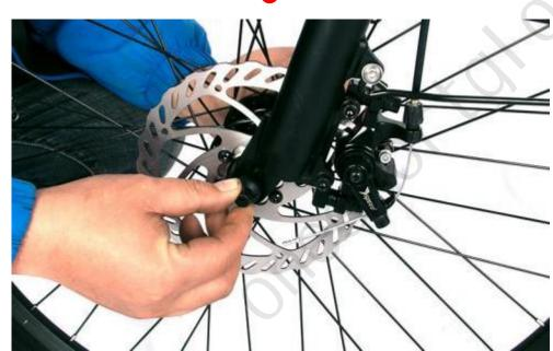
6.Screw on the quick release rod nut as shown in the figure
